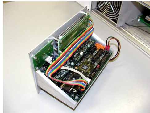
Fig. 7: Rear view of control and protection unit.
