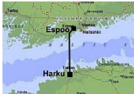
Figure 1: the Estlink cable (Source: ABB)
