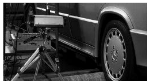
Fig. 6: LDV measurement of a car door
